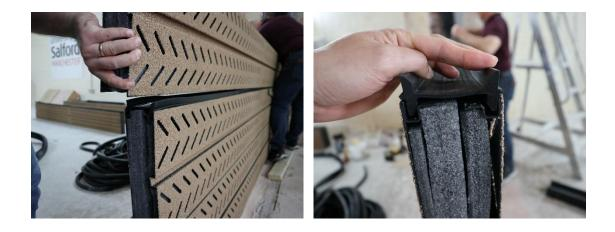
A second, intermediate post was fitted over the ends of the acoustic panels. A shorter, second set of acoustic panels and seals was slotted into the intermediate post, at a slight angle; before a third post was fitted over the end of the assembly, the other recess in this post was filled with a length of timber. The end of the barrier assembly was then moved into its correct position in the test aperture and fixed in place, using L-brackets and screws.
