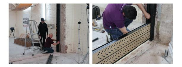
Nine acoustic panels were slotted into the post, with H-section rubber seals between each panel. Each panel was composed of metal rectangle box section planks filled with different types of plastic absorption. The source room face of each panel was pierced with holes, to expose the infill. Both source and receiving room faces were covered with a layer of rubber and cork granules. A single panel was measured to be 2400 mm  $\times$  297 mm  $\times$  75 mm, with a mass of 21.3 kg.
