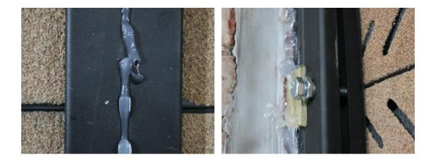
Silicone sealant was used to seal the perimeter of the barrier and the centre seams of the posts, on both source room and receiving room faces. More silicone sealant was used
