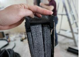
A second, intermediate post was fitted over the ends of the acoustic panels. A shorter, second set of acoustic panels and seals was slotted into the intermediate post, at a slight angle; before a third post was fitted over the end of the assembly, the other recess in this post was filled with a length of timber. The end of the barrier assembly was then moved into its correct position in the test aperture and fixed in place, using L-brackets and screws.
