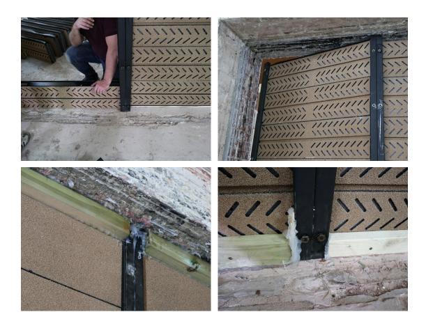
Lengths of timber (screwed to the top panel) were added to close the gap between the barrier and the top of the test aperture, on both source room and receiving room faces. More lengths of timber were screwed to the lowest panel, on the source room face only, to close the gap between the barrier and the base of the test aperture.
