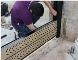
Nine acoustic panels were slotted into the post, with H-section rubber seals between each panel. Each panel was composed of metal rectangle box section planks filled with different types of plastic absorption. The source room face of each panel was pierced with holes, to expose the infill. Both source and receiving room faces were covered with a layer of rubber and cork granules. A single panel was measured to be 2400 mm  $\times$  297 mm  $\times$  75 mm, with a mass of 21.3 kg.
